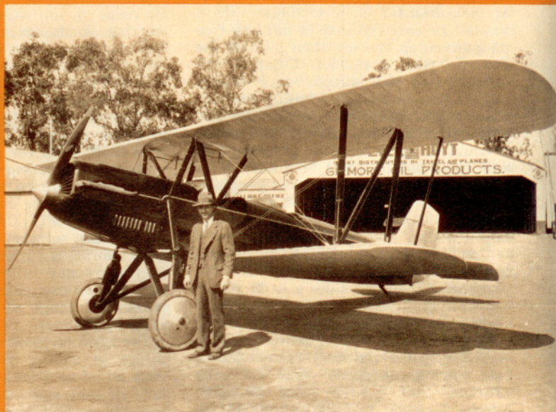
Lloyd Stearman and the C-1 at Venice, Calif., in early 1927. Though using a tailskid, the C-1 had brakes on the wheels, an innovation at the time. Note the aileron strut and the nose radiator, deleted on subsequent Stearman models.
